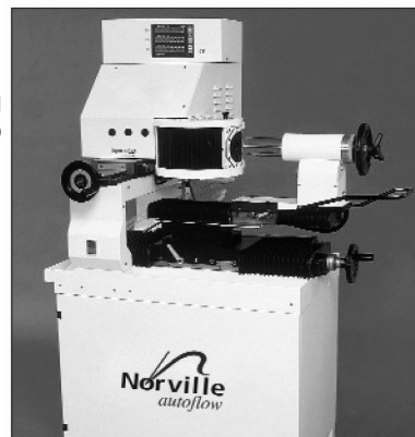
» Figure 7 A lens generator (by courtesy of Norville Autoflow)
