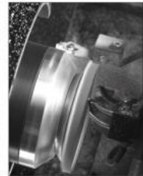
» Figure 12b Finish stage freeform cutting (by courtesy of DAC International)
