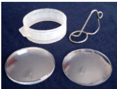
Figure 2 Components used for lens casting - Flexible gasket, spring clip, top & bottom glass moulds
